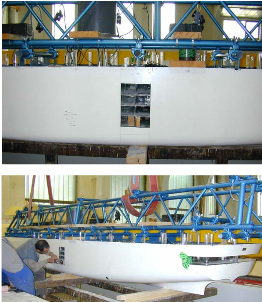
Figure 6: Damaged vessel (STD opened).
