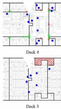
Figure 22 The final equilibrium simulated in time-domain or modelled experimentally, will not always correspond to the statically predicted attitude. The compartment on Deck 3 (marked above-right) floods from the Deck 4 unless damaged directly.
