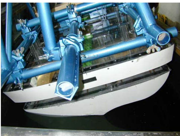
Figure 14 The C1 vessel in heeled condition, some 18deg heel to port side.
