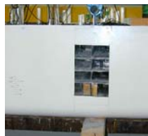
Figure 5 Definition of the "high" damage opening, penetration assumes only external hull damage, with decks remaining intact.
