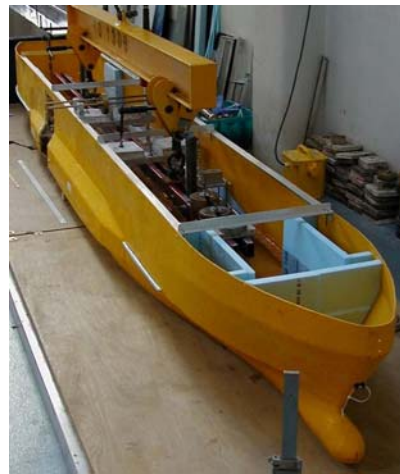
Figure 7: A Typical RORO Model under Construction
